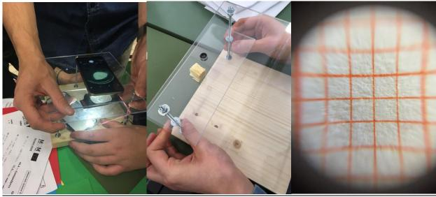
You can use millimiter paper to calibrate by a proportion. See however the distorted image at the boundaries It's fundamental to have the proper light from the bottom. You can regulate the focus by gently turning the screws. The smartphone lens is aligned with the microscope lens. You may also think to enhance the whole system by using one of the many "magnifying lens" app available online.
