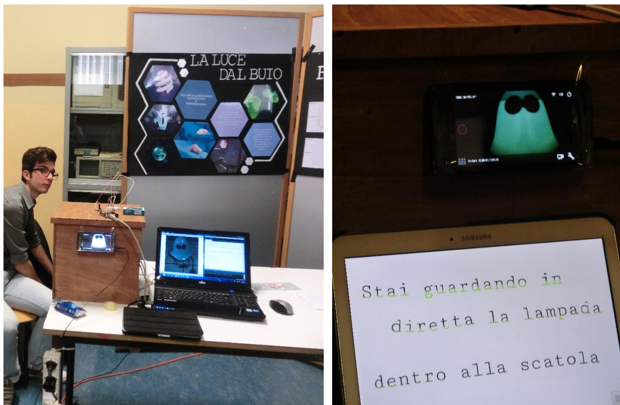
Figura4 - Left: the experimental setup. "The black box" with Arduino on the top. You can notice the photcamera fixed to the front side. Right: detail of the photcamera working .the label reads "you are watching live the photoluminescent lamp inside the box).
